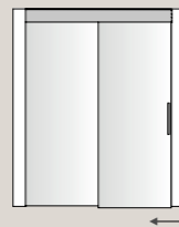
Anta scorrevole e pannello fisso con binario a soffitto / Door and fixed panel on ceiling mounted track
